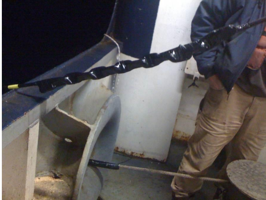
Figure D.22: One of the four lengths of chain used to weigh down the cable.
