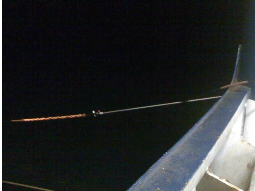
Figure D.20: Hydrophone cable secured by a yale grip to the port sponson
