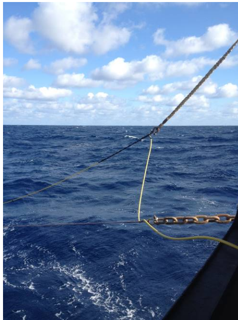
Figure 3. The PAM tow cable connecting to the offset rope via shackle
