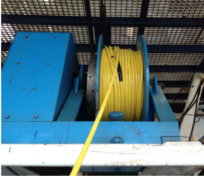
Figure 2. PAM tow cable spooled onto the winch and running aft
