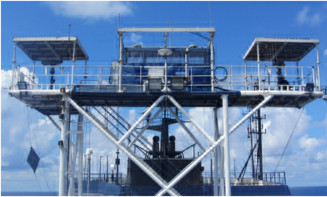
Figure 3. Protected Species Observer observation tower with mounted big-eye binoculars, as seen from the stern of the vessel
