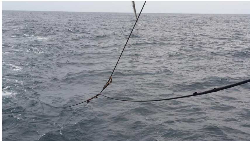
Figure 24: The PAM tow cable connecting to the offset rope via shackle.
