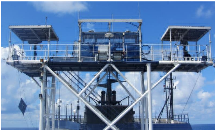
Figure 2. Protected Species Observer observation tower with mounted big-eye binoculars, as seen from the
