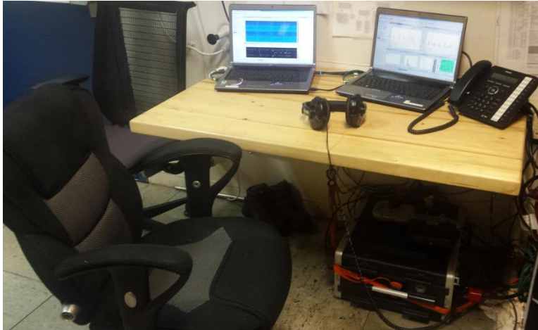
Figure 25: Passive acoustic monitoring station located in the main science lab.
