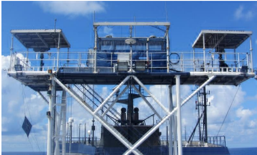
Figure 2. Protected Species Observer observation tower with mounted big-eye binoculars, as seen from the stern of the vessel.
