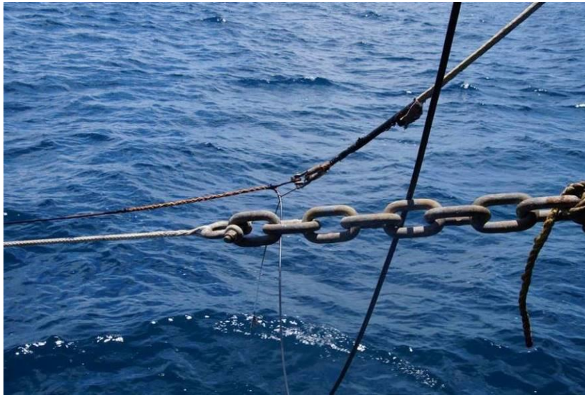
Figure 5: The PAM cable connecting to the offset rope via shackle.
