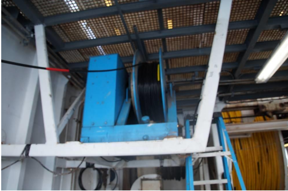
Figure 2: PAM cable spooled onto the winch.
