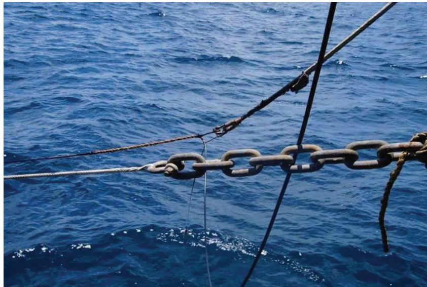
Figure 17: The PAM cable connecting to the offset rope via shackle.
