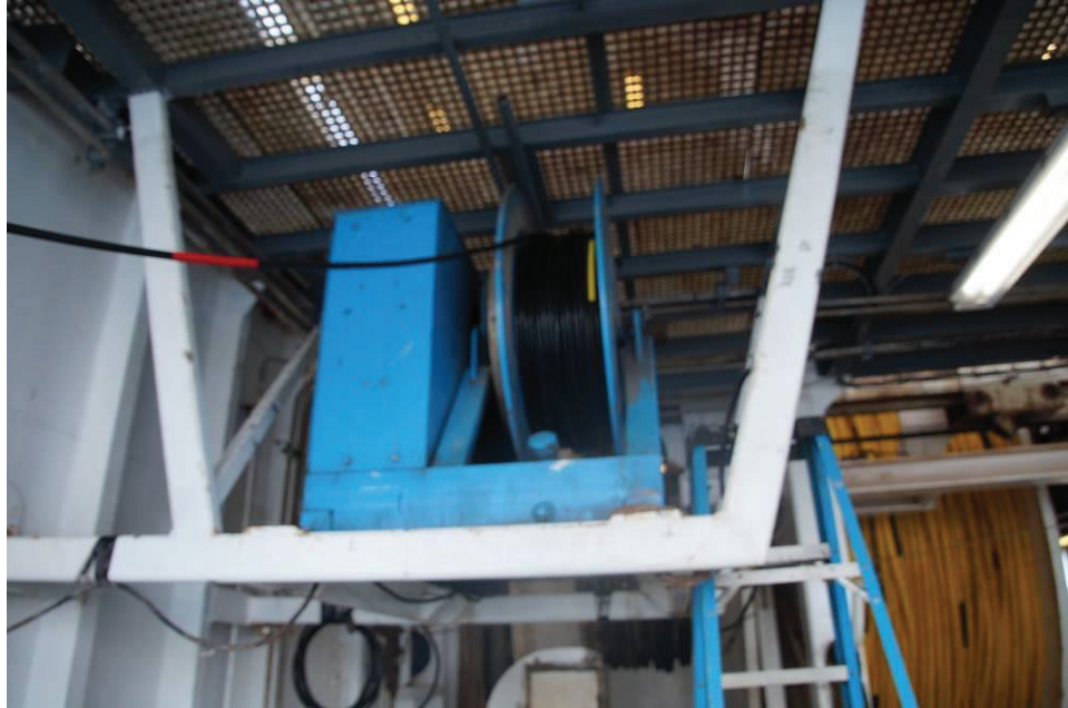
Figure 14: PAM cable spooled onto the winch.
