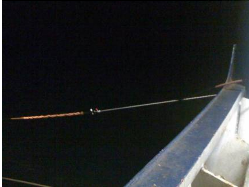
Figure D.4: Hydrophone cable secured by a yale grip to the port sponson.
