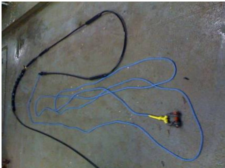
Figure D.5: Rope drogue and first chain weight secured near hydrophone elements.
