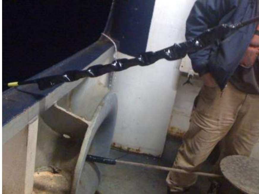
Figure D.6: One of the four lengths of chain used to weigh down the cable.
