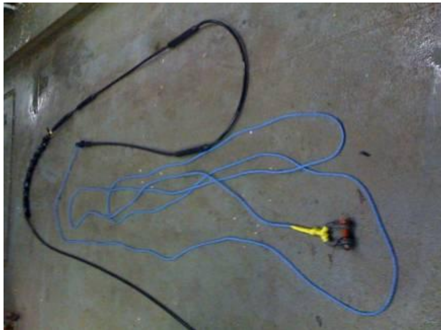
Figure D.20: Rope drogue and first chain weight secured near hydrophone elements.
