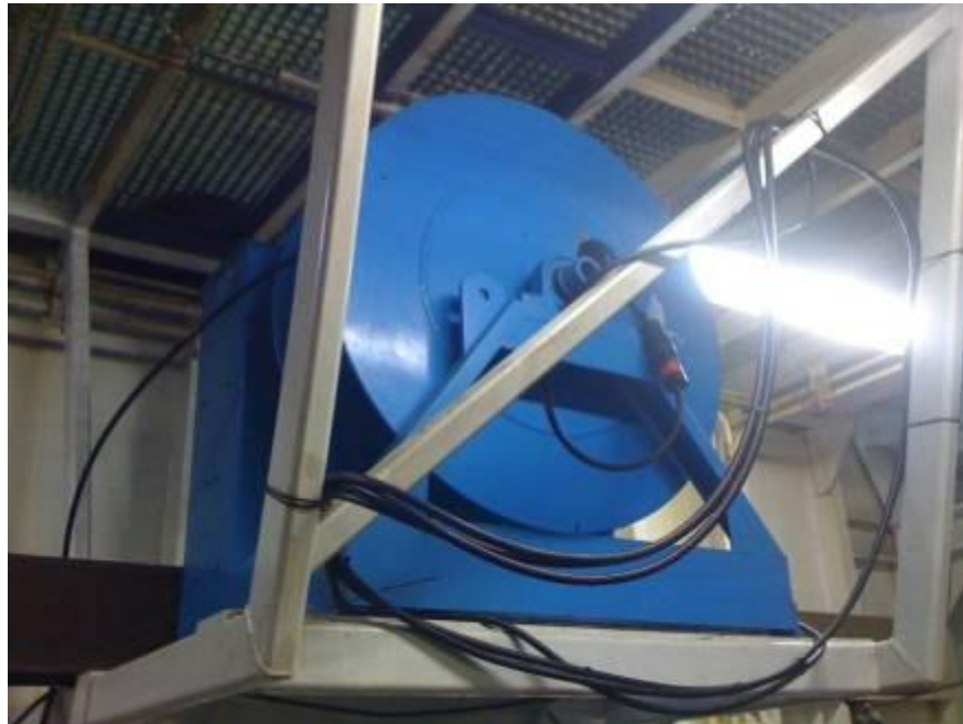
Figure D.18: Hydrophone cable on winch.
