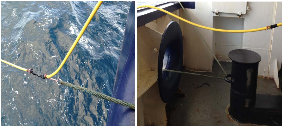
Figure 3. On the left is the PAM tow cable connecting to the towrope via shackle. Right shows PAM going over the stern bulkhead, the towrope tied off to the bitt and threaded through the chalk.
