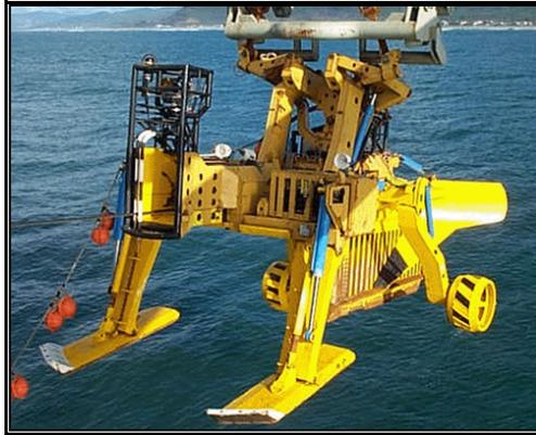
**Figure 2-22. Example of a Submarine Cable Plow**
