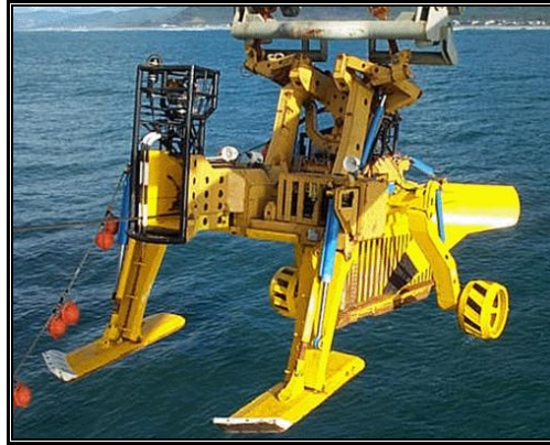
Figure 2-23. Example of a Submarine Cable Plow
