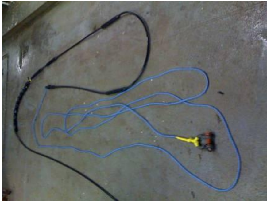
Figure 46 Rope drogue and first chain weight secured near hydrophone elements.
