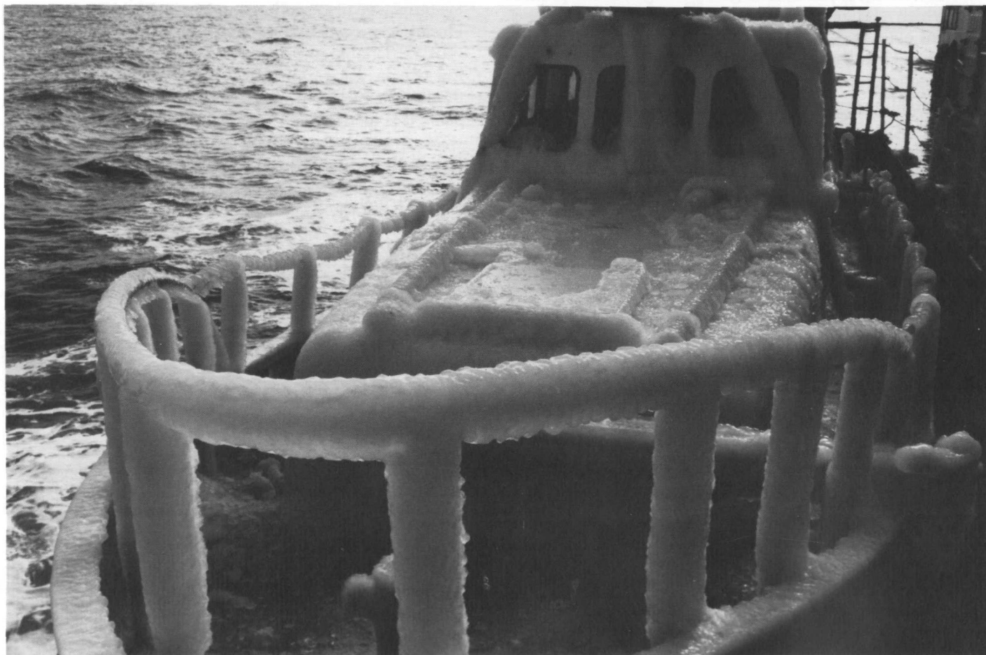
Figure 21. Icing of structures, a hazard to drilling rigs and fishing vessels. (NSF photo by Russ Kinne.)
