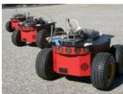
Page 50: These robots are part of the multi-robot testbed and include a custom suite of sensing, computing and communication equipment. Experiments using these robots range from demonstrating control systems that move the robots in formation to a spoken dialogue interface that allows a single operator to command the robots through normal speech.
