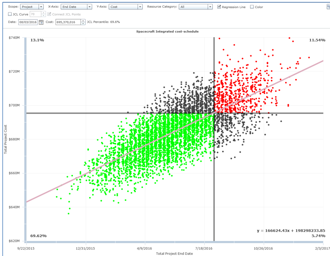
Figure 5.2.8-3 Time-Cost Scatter Diagram: Each data point represents one realization of the simulation
