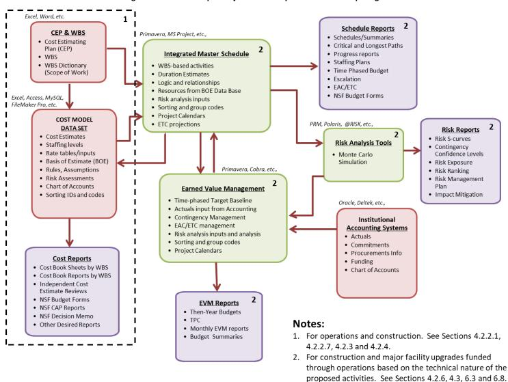
Figure 4.2.2-1 Sample Project Control Systems Relationship Diagram
